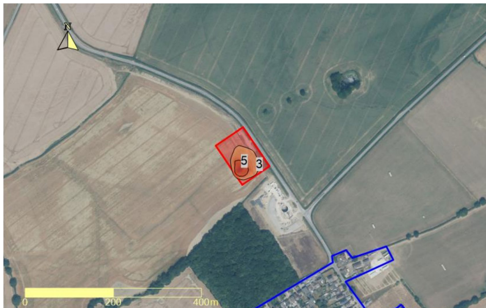
Figure 12 – Results of the dispersion model sensitivity analysis – double emissions
